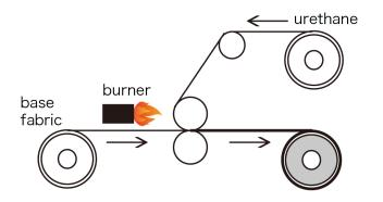
Flame is fire and lamination is the uniting of separate layers into a whole. Flame lamination processing is the method of using flame to laminate. Lamination is accomplished by applying flame to the surface of a soft urethane foam and affixing cloth, film or other base material to the melted section of the foam.
